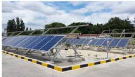
Outdorr bench for PV modules performance evaluation
